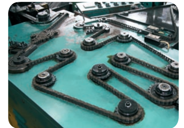
Automated chain assembly to ensure proper fits and tolerances are met.
