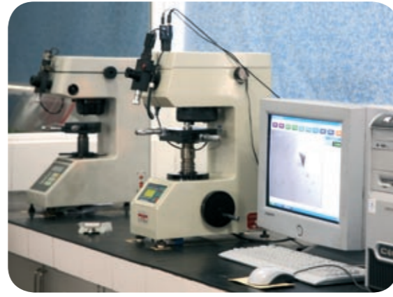
Microhardness testing equipment where batch tests are done to ensure hardness is within specification
